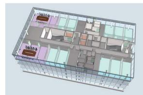
With Desigo TRA, flexibility means being able to adapt the building's floor plan and partitioning of individual rooms both quickly and easily through the sophisticated segment concept – without changing the electrical and HVAC installation. The result is a lower initial expenditure and lower costs in the basic configuration as well as complete freedom to add functional expansions when adding tenants.
